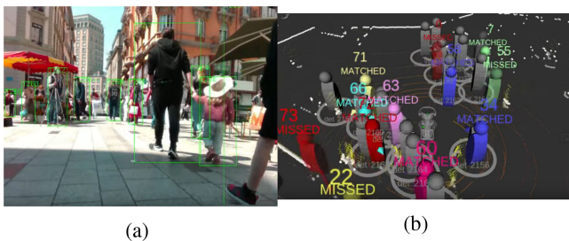
Fig. 23. (a) Camera and the LIDAR of the robot are interpreted by the (b) detector, which is used for the obstacle avoidance algorithm. (a) Camera view. (b) Detector interpretation.
