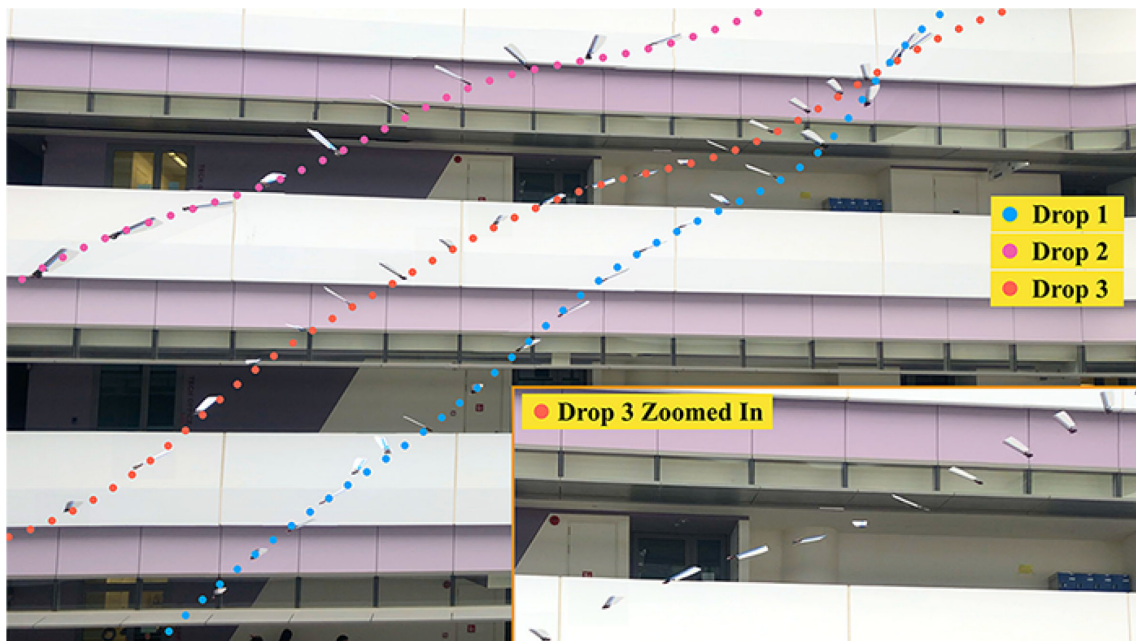
Fig. 15. dSAW prototypes were dropped by hand and square cyclic control was applied shortly after. Still frames of dSAW were extracted and displayed in sequence to show its pose. An average glide angle 0.5044 rad ( 28.9^\circ ) was achieved. Lower right corner shows a close up of Drop 3. Each frame was captured 0.25 s apart, hence, dSAW had rotated slightly more than 1 rotation between each frame.
