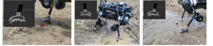
Fig. 9. Pose reconstruction of SoftFoot-Q on ANYmal. The shape of the foot is estimated by the software even under water.
