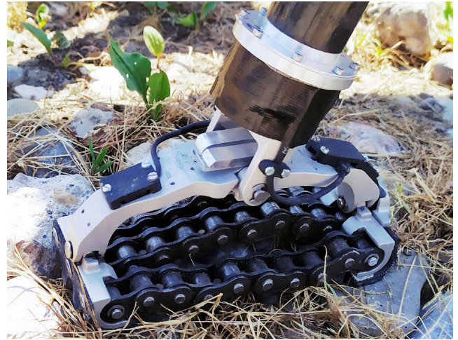
Fig. 1. SoftFoot-Q, a passive adaptive foot designed for quadruped robots.
