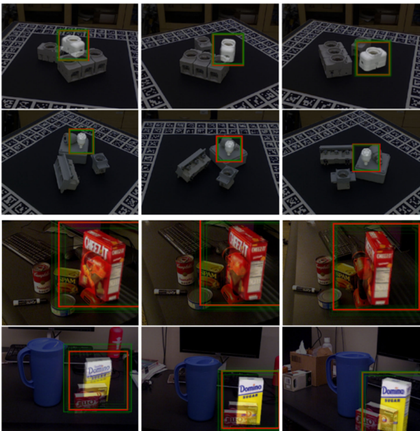
Fig. 7. Visualization of estimated poses on the T-LESS dataset (first two rows) and the YCB Video dataset (last two rows). Ground truth bounding boxes are red, green bounding boxes are particle RoIs, and the object models are superimposed on the images at the pose estimated by PoseRBPF.
