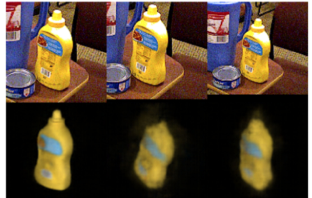
Fig. 5. Visualization of reconstruction of the RoIs from autoencoder. Left is the ground truth RoI. The other two columns show the reconstruction with shifting and scale change. As shown, the reconstruction quality degrades with deviations from the ground truth RoI. In this example, the similarity score drops from 0.91 to 0.62 and 0.72 with the deviations, respectively. This property makes the autoencoder a suitable choice for computing the observation likelihood.
