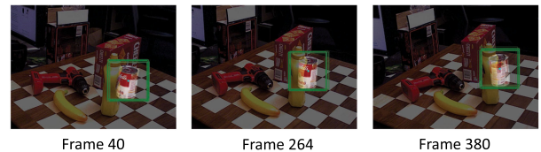
Fig. 11. Example of tracking failure due to occlusion. The plot shows that the maximum similarity (blue curve) decreases with increasing occlusion (red curve). In our implementation, the system determines tracking failure when the maximum similarity is lower than 0.6. Therefore, our system can handle about 65% occlusion before failure in this example.
