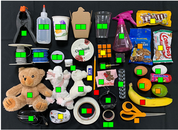
Fig. 17. Thirty-six objects used in our experiments. Colored boxes on each object indicate the number of successful grasping out of three trials: green (3/3), yellow (2/3), orange (1/3), and red (0/3). Objects with two colored boxes were tested in two different orientations.
