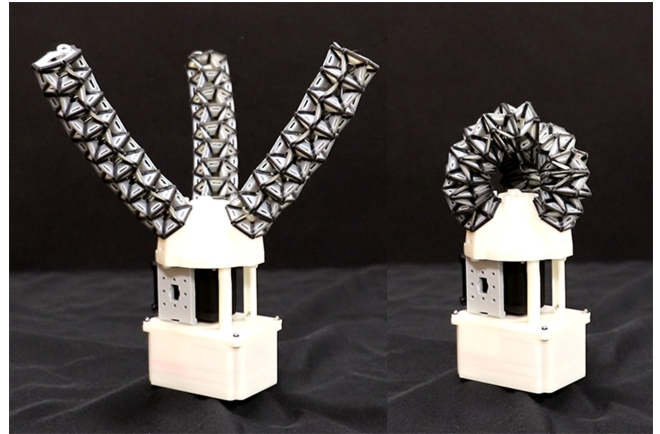
Fig. 1. Underactuated cable-driven robotic gripper with three compliant fingers fully open (left) and closed (right).
