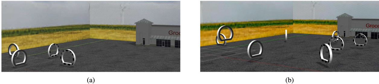
Fig. 4. Illustration of the simulated tracks. The small track (a) consists of four gates and spans a total length of 43 m. The large track (b) consists of eight gates placed at different heights and spans a total length of 116 m.
