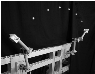
Fig. 18. Experimental setup with two symmetric robots acting in a common vertical plane. Each robot has two actuated rotational degrees of freedom and is capable of performing both the throwing and the catching task, without change of hardware.
