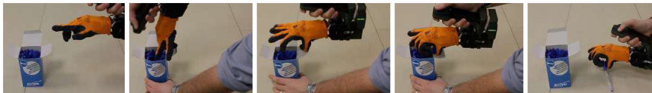
Fig. 18. SoftHand 2 extracts a pen from its package, by relying on the preshaping ability provided by the second DoA.
