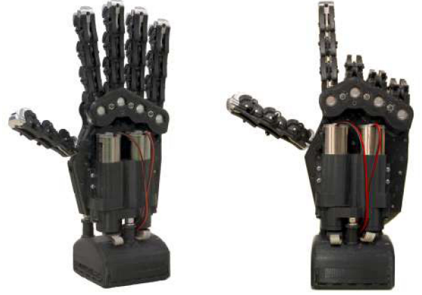
Fig. 6. Pisa/IIT SoftHand 2 evolves Pisa/IIT SoftHand through the introduction of an additional DOA, powered by a friction-based transmission system. The hand design is self-contained, including the whole actuation system, sensors, power, and control electronics.
