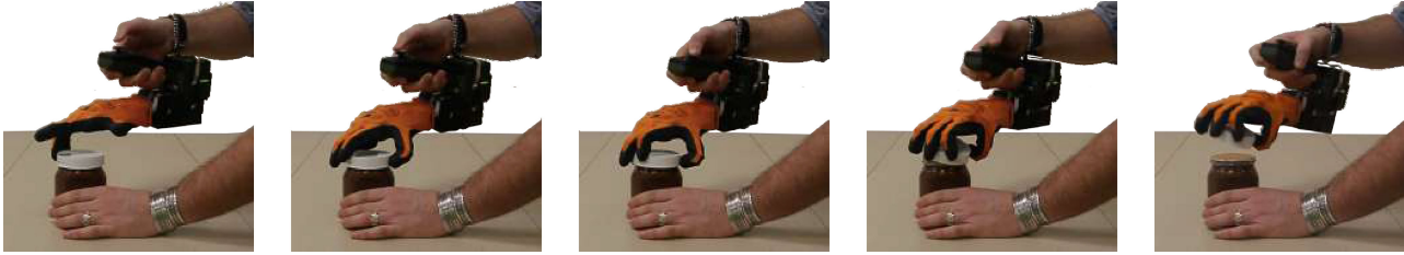
Fig. 20. Example of in-hand manipulation. We can use SoftHand 2 for opening a jar without main compensations on the wrist level.
