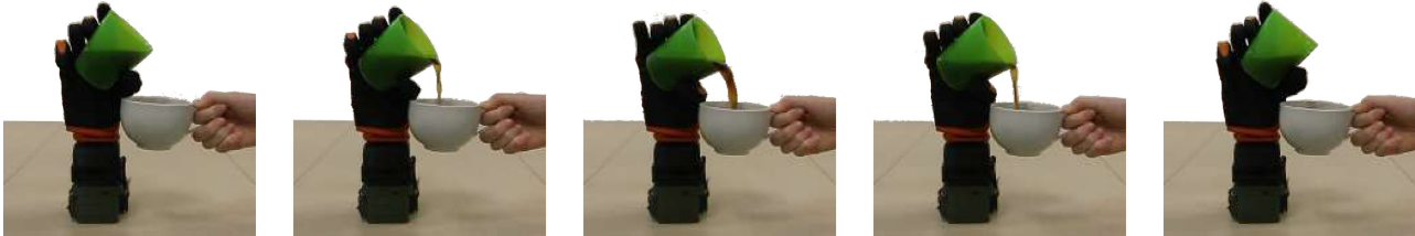
Fig. 21. Example of in-hand manipulation. Following a feedforward input, SoftHand 2 pours coffee from a cup to another.
