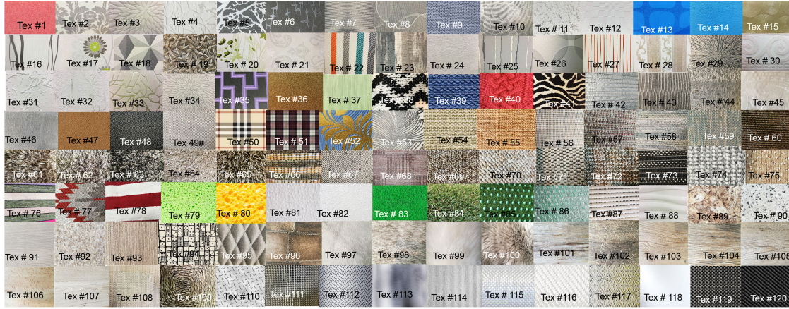
Fig. 3. Selected experimental materials consist of 120 different natural and synthetic textures with uniform (regular) and nonuniform (irregular) structures including papers and vinyl wallpapers (Tex.#1-Tex.#37), textiles (Tex.#38-Tex.#57), carpets and mats (Tex.#58-Tex.#78), foams and sponges (Tex.#79-Tex.#82), fibers (Tex.#83, Tex.#84), PVC and rubber type surfaces (Tex.#85-Tex.#95), leathers and furs (Tex.#96-Tex.#100), wooden surfaces (Tex.#101-Tex.#109), metal surfaces (Tex.#110-Tex.#113), fiberglass and glass surfaces (Tex.#114-Tex.#118), and carbon sheets (Tex.#119, Tex.#120). All materials were acquired from Bauhaus.
