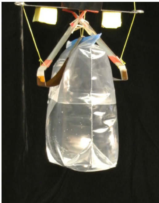
Fig. 1. Flexible shear-activated gripper holds a water-filled bag. Load tendon is at center; outer tendons release the adhesive film.
