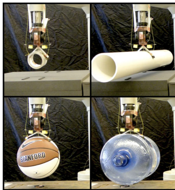
Fig. 28. Grasping tasks with a curved surface gripper implemented on a robotic arm. The gripper is shown lifting (clockwise from upper left): packing tape, 3.5-kg PVC tubing, empty 5-gal water jug, and a regulation basketball.
