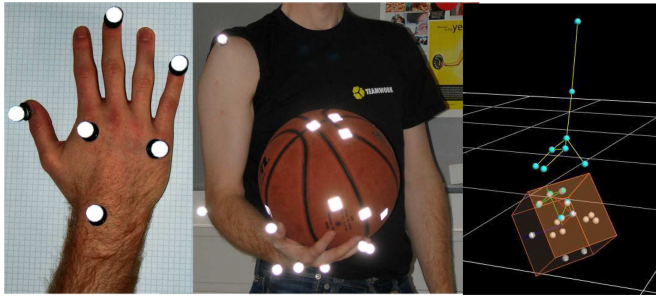
Fig. 25. Setup and marker positions for the human dribbling experiments (left and center), sample data of a tracked pose visualized in ViconIQ (right).
