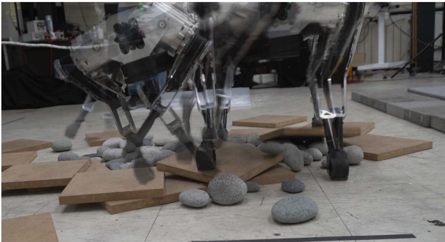
Fig. 1. Example scenario when static contact assumption of the foot is violated. A strong pulling force is applied to the quadruped robot Hound [3] while walking on a terrain made with moving wood piles and pebbles.
