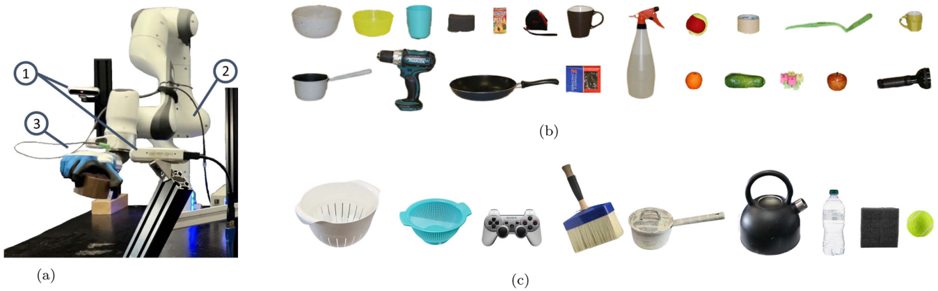
Fig. 9. (a) Experimental setup and complete set used for the experimental validation. (b) 30 objects, of which 21 are the ones used in [19]. (c) Nine additional objects; from left to right: Big Colander, Small Colander, Controller, Brush, Pot, Boiler, Bottle, Foam Brick, and Tennis Ball. (a) Experimental Setup. (b) Objects from [19]. (c) Additional objects tested.
