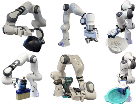
Fig. 1. Ability to grasp previously unseen objects with different grippers; adapting to imperfectly known, highly dynamic, and unstructured situations is crucial to enable general-purpose robots to be effective in a large field of use cases.
