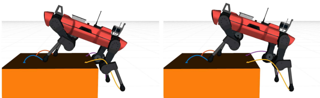
Fig. 8. ANYmal stepping up a box of 35 cm. Left: Without considering knee collisions. Right: Knee collision included in the optimization.
