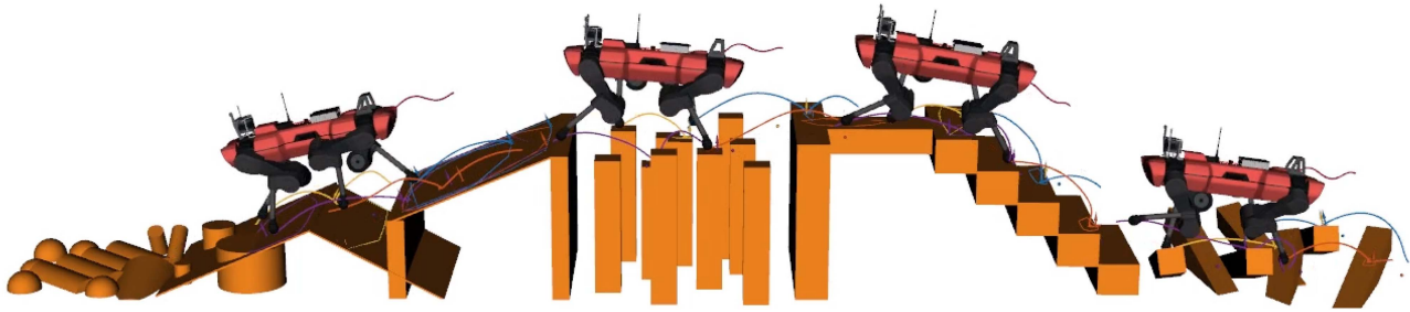
Fig. 13. ANYmal traversing an obstacle course in simulation (left to right). Snapshots are shown for a traversal with a trotting gait at 0.8 \text{ ms}^{-1} . The MPC predictions are shown for each foot and for the torso center. For all contact phases within the horizon, the convex foot placement constraints are visualized.
