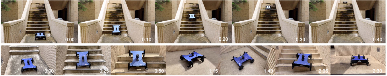
Fig. 24. Time-lapse sequence images from two separate trials of stair climbing on a U-shaped double staircase [see Fig. 23(a)] using the embedded algorithm presented in the Appendix.
