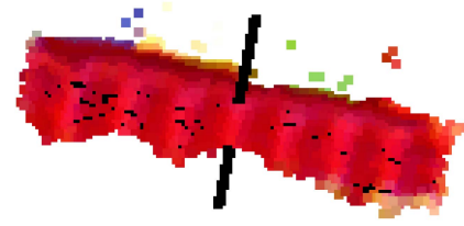
Fig. 7. Example of a grasp on a red Lego block. The black line shows where the robot finger tips are positioned when grasping (the black line goes through finger tip positions). The robot tries to grasp a narrow part of the point cloud. In detail, the grasp is based on the second PCA eigenvector of the point cloud projected on the 2-D plane going through the wrist of the robot (not shown).
