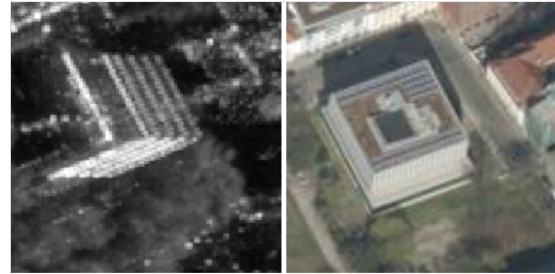
Fig. 1. Simple detached multistory building as (Left) SAR amplitude image and (Right) optical photograph.
