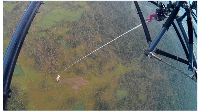
Fig. 2. Photograph of the fluxgate magnetic tensor gradiometer towed by the helicopter in the flight experiment.
