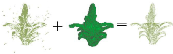
Fig. 6. Model merging. (a) The original point cloud data consisting of outliers, (b) the PPR representation containing unverified voxels, and (c) the merged model with the removal of outliers.
