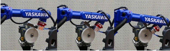
Fig. 12. Image sequence showing the task execution without processing the demonstrated motion with the proposed redundancy resolution scheme. The execution failed due to the violation of joint limits.
