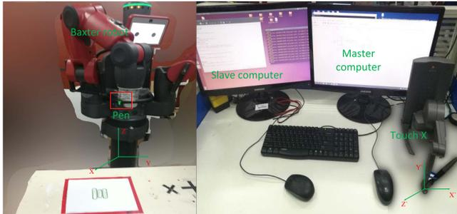
Fig. 9. Experimental setup for a drawing task.
