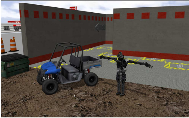
Fig. 13. The DARPA Robotics Challenge (DRC) used CloudSim, an open-source Cloud-based simulation platform for testing the performance of the Atlas humanoid robot (shown) on a variety of disaster response tasks [5], [7]. The Cloud permits running interactive, real-time simulation tasks in parallel for purposes such as predicting and evaluating performance, validating design decisions, optimizing designs, and training users. This competition also resulted in enabling sharing of robotics research efforts. (Image reproduced with permission.)
