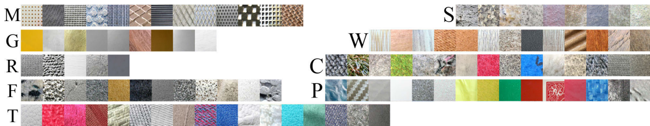
Fig. 4. The online LMT108 dataset [12] covers 108 surfaces from nine material categories: (M) thirteen meshes, (S) nine stones, (G) nine glossy materials, (W) thirteen wooden materials, (R) five rubbers, (C) fifteen carpets, (F) twelve foams, (P) fifteen plastics and papers, and (T) seventeen textiles and fabrics.
