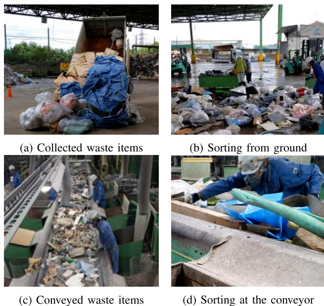
Fig. 1. Images showing current processes of sorting mixed industrial waste. (a) Collected waste items are unloaded from a truck, (b) manual sorting of the mixed industrial waste from the ground, (c) collected waste items on a conveyor, and (d) manual sorting at the conveyor.
