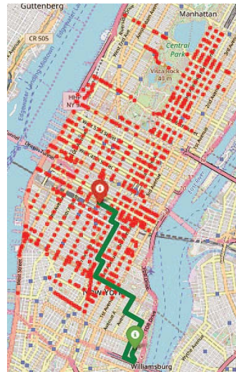
Fig. 2: A spoofed path example in Manhattan and the escape destinations generated for that single spoofed path. Our algorithms generate 100 distinct spoofed paths for a given start and end location, allowing an adversary to undetectably reach an even larger set of escape destinations.
