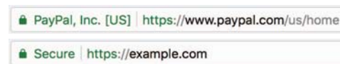
Fig. 2. The Chrome Extended Validation certificate UI (top) and default UI shown for regular HTTPS certificates (bottom).
