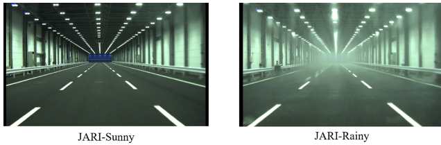
FIGURE 4. Scene examples of the JARI dataset for radar translation. From left to right, they depict sunny and rainy data for the JARI dataset. The JARI dataset is collected with adjusted precipitation levels.
