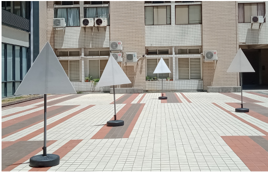
FIGURE 9. The targets are placed in an open area. Multiple targets are used to collect more target measurements and accelerate the calibration process.
