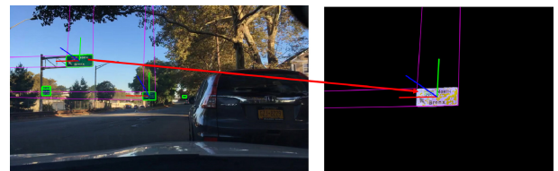
FIGURE 6. Visually estimating the 3D direction of traffic signs from a 2D image mask.
