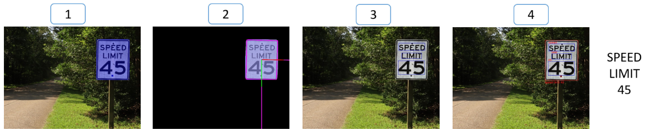
FIGURE 5. Step-by-Step Example output: 1) displays the results after sign detection (sign instance masks, shown in the blue shaded region); 2) shows the outcomes of sign relevance, with the orientation of each extracted sign indicated by green and red line segments (green represents the y-directional eigenvector, and red represents the x-directional eigenvector); 3) illustrates the individual text extractor instances; and 4) demonstrate the processing of individual instances for recognition and the resulting text recognition outcomes.
