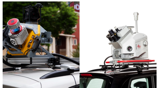
FIGURE 6. Two examples of MMS: Trimble MX9, Leica Pegasus Two Ultimate. Courtesy: Trimble and Leica-Geosystems websites.
