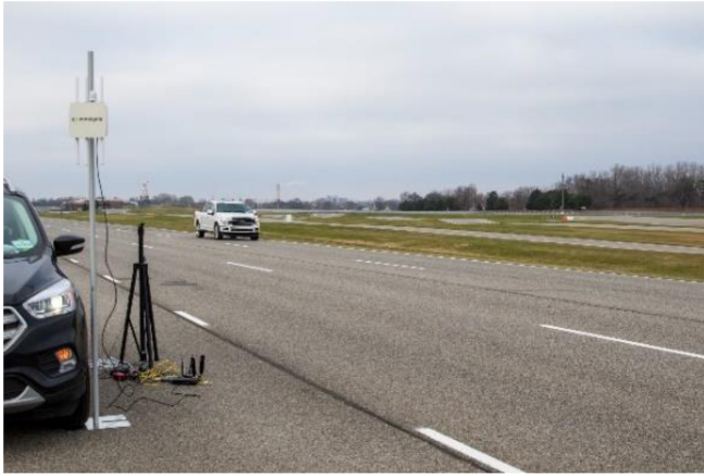
FIGURE 2. Showing Vehicle and Road-Side-Unit setup on Test Track.
