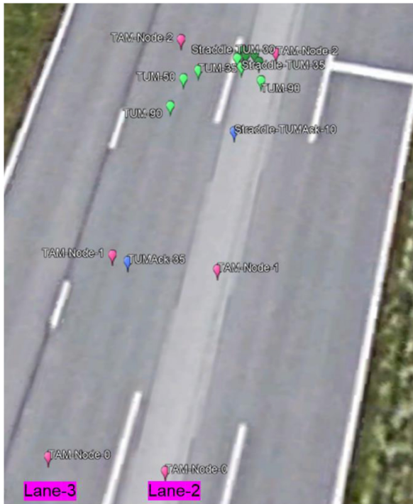
FIGURE 15. Another Closer View of GPS KML Positioning Points of TUM Trigger at Toll Zone.
