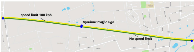
FIGURE 6. Visualization of dynamic traffic sign information: combined vehicle and infrastructure perspective. Blue points indicate a dynamic traffic sign with its infrastructural information (e.g., last update). Continuous lines represent the allowed speed on the given lane (yellow - 100 kph speed limit, green - no limit).
