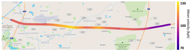
(a) Visualization of the vehicle perspective. The mean velocity measured by the loop detectors is displayed along the course of the road.
