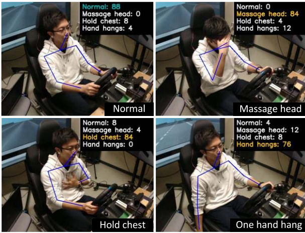
FIGURE 9. Output of posture classification system. The percentage shows the number of the closet training data out of k ( k=30 ).
