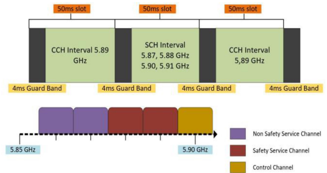
FIGURE 3. Alternate channel access of ETSI ITS-G5 standardization.
