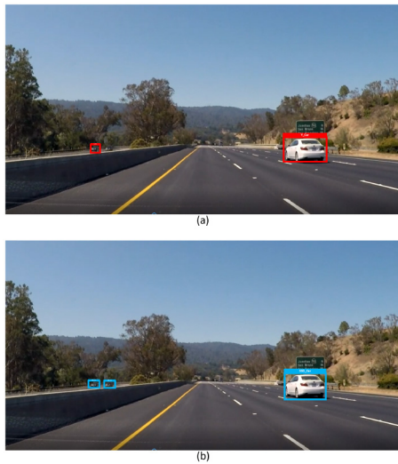
FIGURE 10. Snapshots taken at the same instant showing the detected vehicles using (a) YOLO, and (b) SSD.
