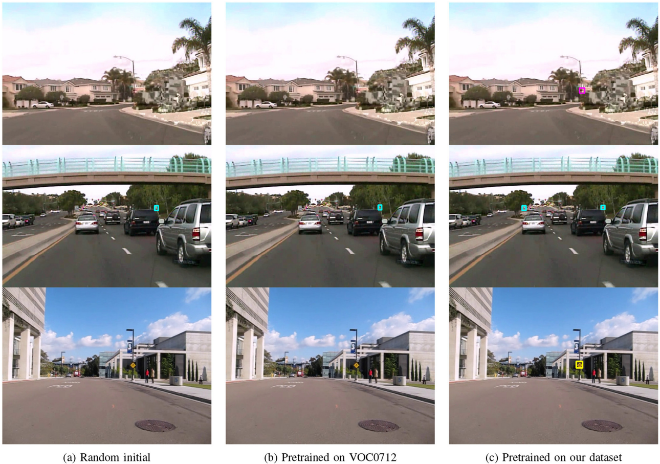
FIGURE 7. Qualitative results on LISA varying pretrained dataset. Mandatory, prohibitory, and warning signs are marked with cyan, magenta, and yellow bounding boxes, respectively. The network pretrained on our dataset can be finetuned to detect U.S. traffic signs. It is more effective in the detection of small traffic signs, as compared to other detectors.
