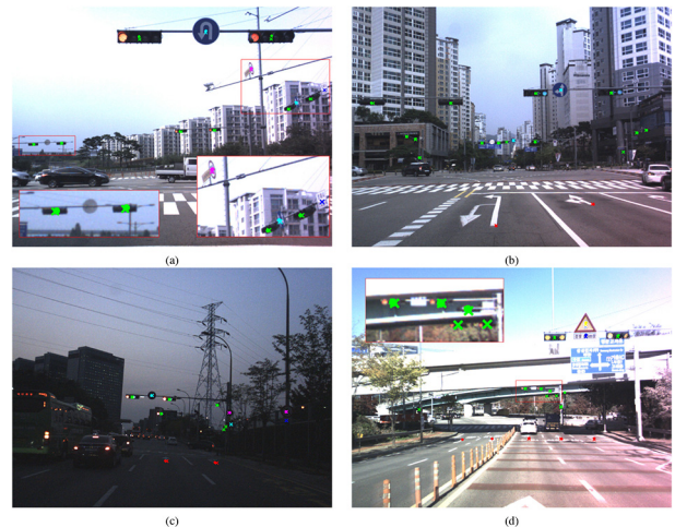
FIGURE 5. Qualitative results of the traffic landmark reference point detection. Warning, prohibition, mandatory, and supplementary signs, traffic light, and road marking are marked with yellow, magenta, cyan, blue, green, and red circles, respectively. Ground truth landmarks are marked with crosses. Note that the reference point of road marking is the bottom right corner of the marking. Our detector successfully localizes the reference points of the traffic landmarks of various scales, in different directions, and under different lighting conditions.
