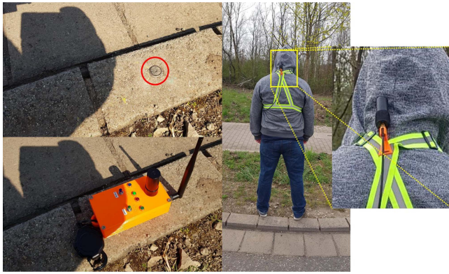
FIGURE 10. Setup to measure accuracy and precision; upper left: GRP; lower left: GMD on GRP; middle: MPD over GRP; right: Detail on antenna/
