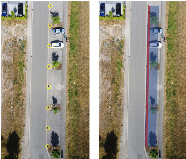
(a) cone positions marked with yellow circles (b) calculated area based on cone positions
