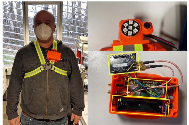
FIGURE 8. MPD; left: attached to a vest; upper right: warning device; lower right: inside of the MPD: a) GNSS receiver; b) Microcontroller; c) battery and charge controller (see Figure 7).
