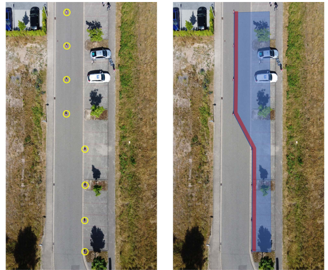
(a) cone positions marked with yellow circles (b) calculated area based on cone positions
