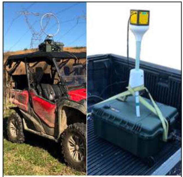
FIGURE 6. Example of the EPRI PREMS II system mounted in the bed of an ATV.
