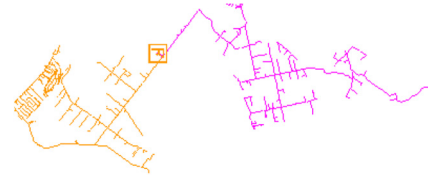
FIGURE 3. Topology of the two connected feeders.
