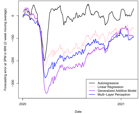
FIGURE 5. Evolution of the forecasting error for the different models introduced in Section III trained on the data up to January 1, 2020.
