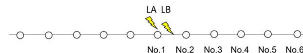
FIGURE 2. Line topology and lightning strike locations LA at pole No. 1 and LB 20 m away from pole No. 1.
