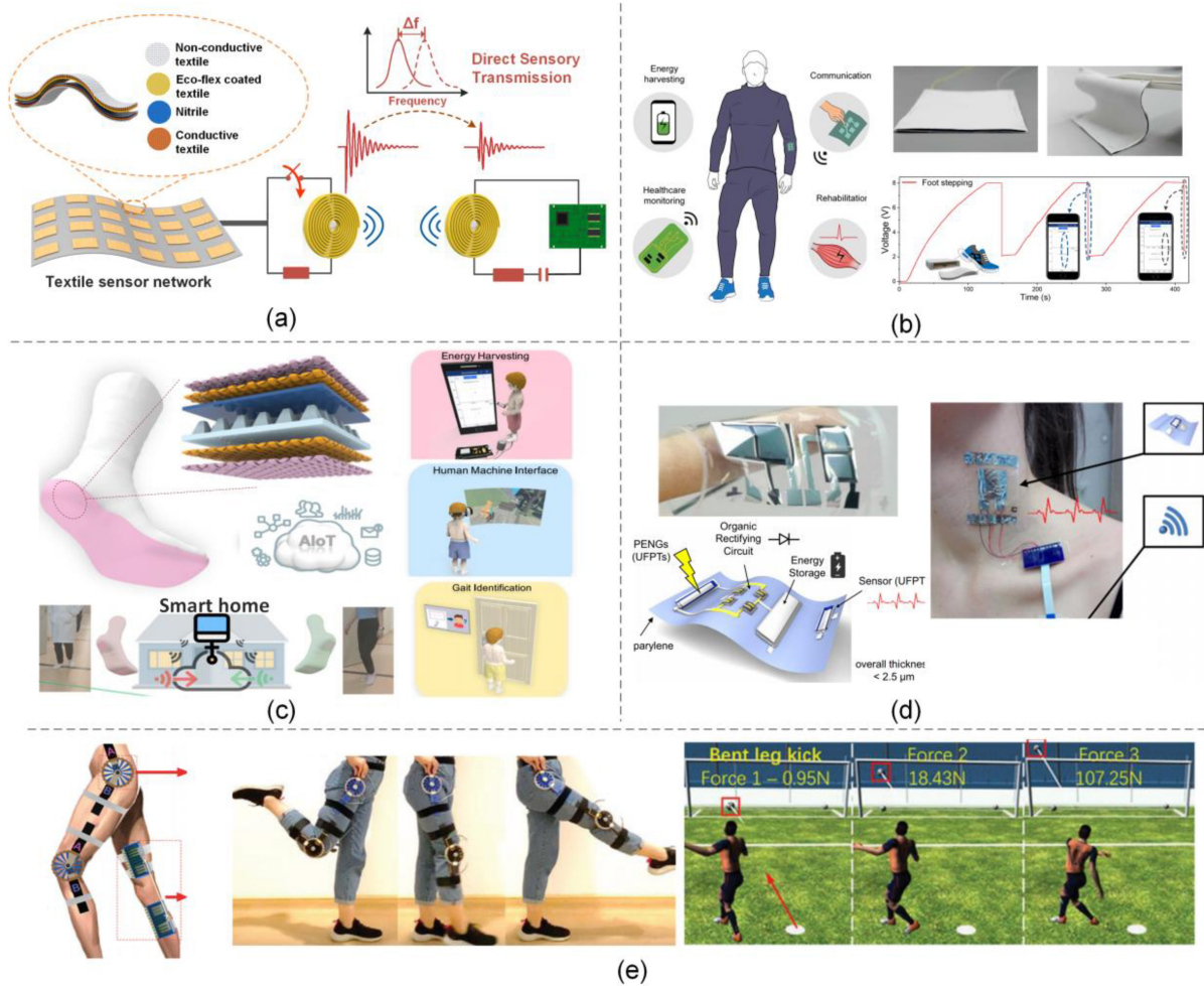
FIGURE 4. Self-sustainable and wearable sensing systems. (a) A battery-free self-powered wireless sensor node based on a triboelectric direct sensory transmission mechanism [167]. (b) A self-sustainable wearable textile system for next-generation healthcare applications [168]. (c) A deep-learning enabled smart sock based on textile-based triboelectric sensors for gait analysis and human-machine interfacing [93]. (d) An imperceptible sensing and energy harvesting patch based on ultra-flexible ferroelectric transducers and organic diodes [169]. (e) A 3D-printed motion capturing and energy harvesting hybridized lower-limb (MC-EH-HL) system for rehabilitation and sports applications [170].
