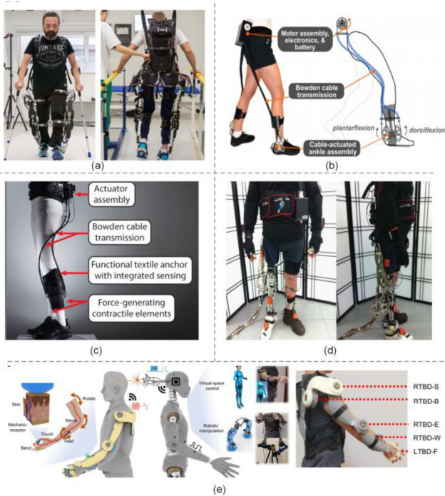
FIGURE 6. Lower-limb exoskeletons and prosthesis to restore or augment walking performance. (a) A modular exoskeleton for incomplete and complete spinal cord injured individuals [198]. (b) An untethered exoskeleton with real-time biofeedback for walking performance augmentation in individuals with cerebral palsy [104]. (c) A soft robotic exosuit for post-stroke gait assistance and rehabilitation [105]. (d) A powered above-knee prosthesis with volitional control for gait assistance of above-knee amputees [106]. (e) A exoskeleton manipulator with bidirectional triboelectric sensors for enhanced multiple degree of freedom motion sensing [199].
