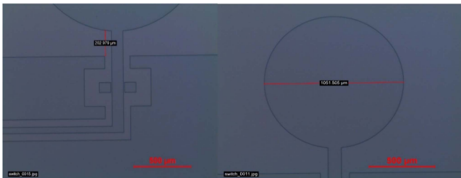
FIGURE 4. Patterned wafers (a) proposed switch region (b) antenna circular patch region.
