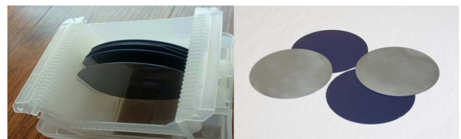
FIGURE 2. Silicon wafers, (a) cleaned wafers (b) single side polished wafers.
