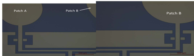
FIGURE 23. Proposed antenna structure (a) patch A (b) patch B.
