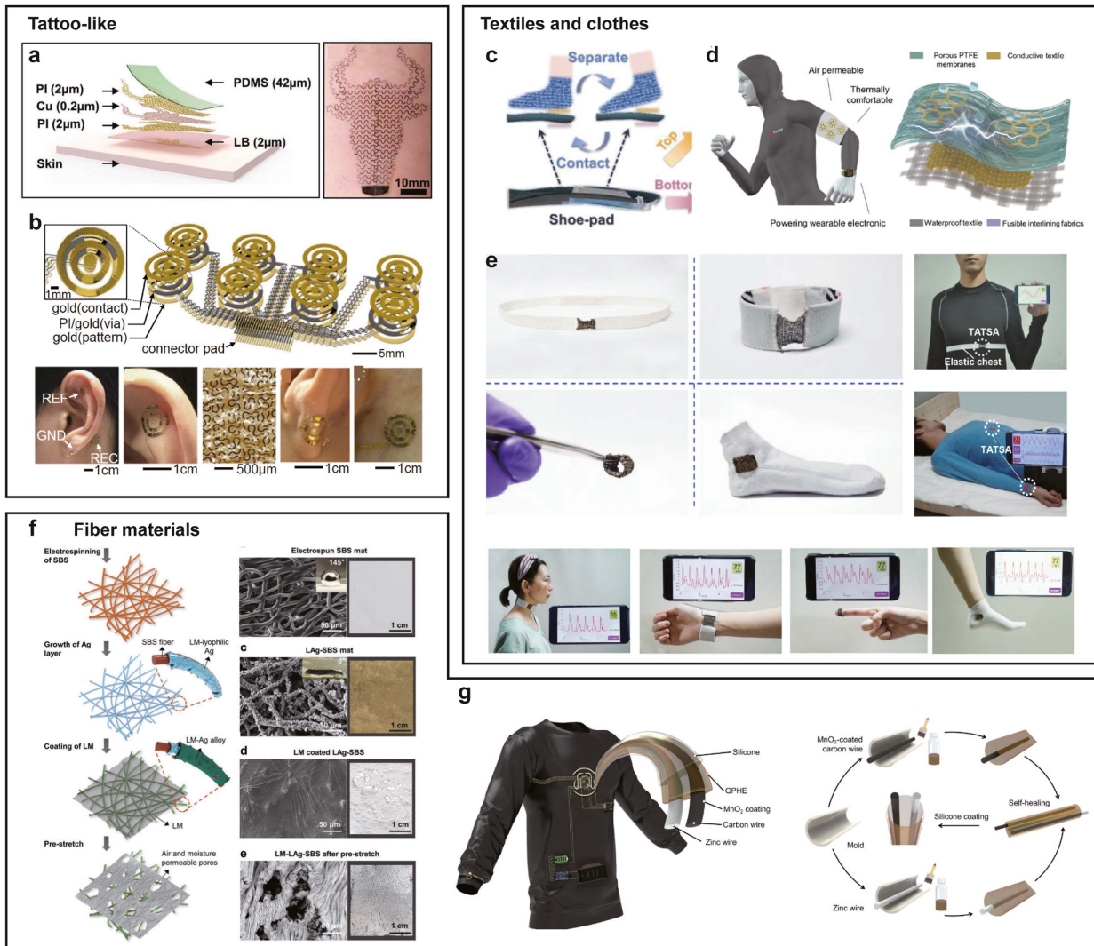
FIGURE 5. Comfortability designs in skin electronics. (a) Tattoo-like ultrathin triboelectric nanogenerators (TL-TENG) [55]. (b) Ultrathin electroencephalography (EEG) electrodes as brain-computer interface [56]. (c) Nanofiber composite based energy harvester of shoepad for collecting energy from walk and running [57]. (d) Textile-based skin electronics as energy harvesting through raindrops [58]. (e) Textile-based triboelectric sensor with good washability [59]. (f) Liquid metal - superlyophilic and stretchable fiber based material for wearable device design [60]. (g) Fiber-based Zn/MnO 2 battery with high cycling stability [61].
