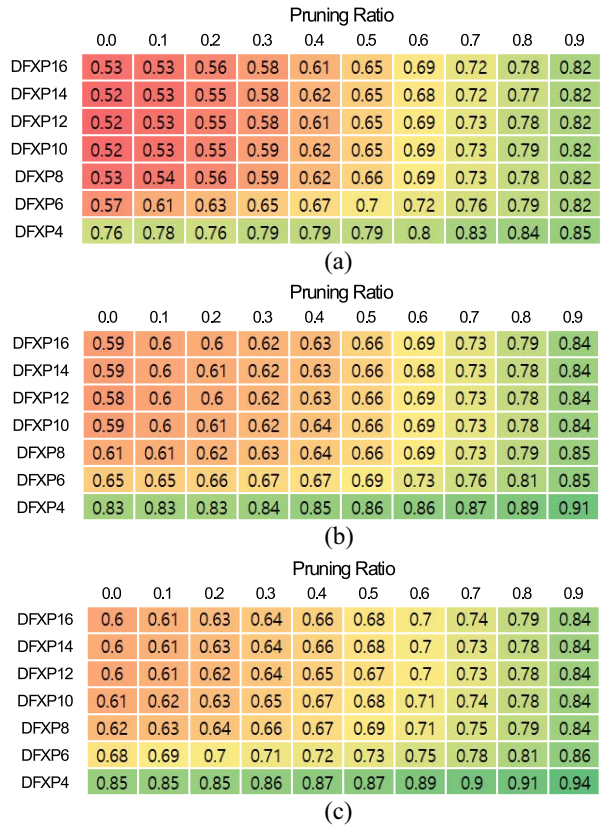
FIGURE 10. IA sparsity of ResNet-9, ResNet-18, and ResNet-34. (a) IA sparsity of ResNet-9 after retraining for pruning and quantization. (b) IA sparsity of ResNet-18 after retraining for pruning and quantization. (c) IA sparsity of ResNet-34 after retraining for pruning and quantization.
