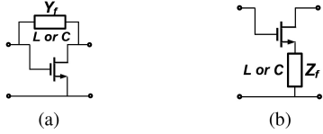
FIGURE 19. Two basic types of embedding network for a transistor (a) Y-embedding (b) Z-embedding.
