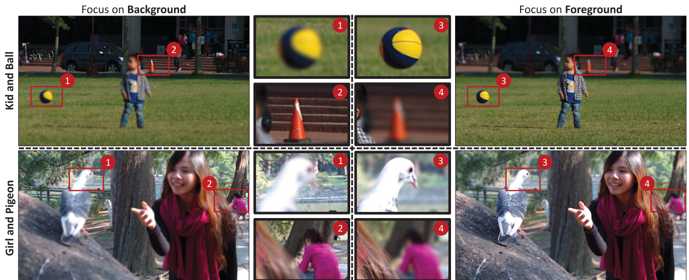
FIGURE 17. Realistic refocusing results generated by the test chip. The target focusing depth can be configured through the programmable parameters of the chip. Objects will be blurred if they are not in the target focus depth (number 1 and number 4 for example).
