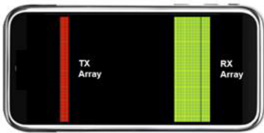
FIGURE 17. Reflection mode imager using arrays of TX and RX pixels incorporated on a smartphone.
