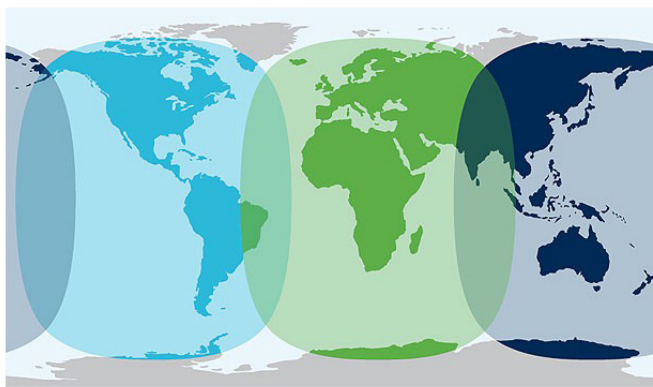
FIGURE 1. Three GEO satellites can almost cover the whole globe [13].
