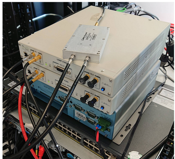
FIGURE 8. Two Ettus X310 URSPs functioning as both the gNB and the UE in the NTN demonstration.
