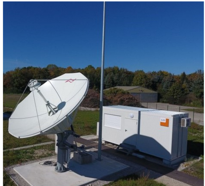
FIGURE 7. GEO transmissions with a 4.9 m satellite antenna and co-located gNB and UE in the laboratory building.
