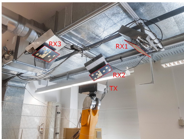
FIGURE 5. Hardware setup consisting of a 24 GHz CW-transmitter (TX) mounted on a precise robotic arm, as well as three receivers (RX) mounted on the ceiling.
